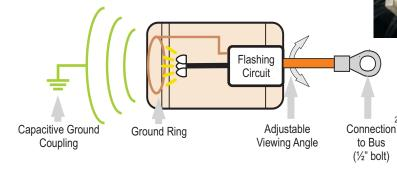
Capacitive coupling between the R-1VH / R-1VL and earth ground provides a means of completing the flashing circuit without a hardwired ground connection. This allows for enough energy to flash the LEDs.
