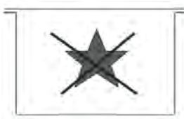
Ex-e prevents the possibility of excessive heat, arcs or sparks from occurring on internal or external parts of the apparatus in normal operation.
