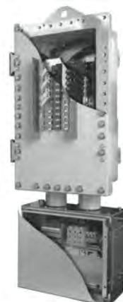
PowerPlus™ panelboards are fully wired for breakers and additional spaces. Factory-sealed Multi-Sleeve Modules™ are removable, so conductors can be replaced and retain third-party approval.
