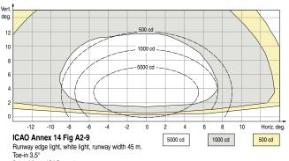
Dotted lines, ICAO requirements The lower parts of the actual light distribution curves
