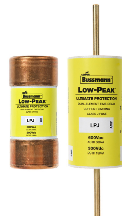
Figure 41: Low-Peak Class J fuses achieve rejection by their unique physical size that is unlike other CSA class fuses.
